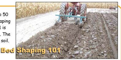
The single-toolbar 3101 is basic. With little practice, operators can quickly gauge cutting depth with the tractor hitch. Bed height depends on depth of cut. The doubletoolbar 3201 features gauge wheels for drop-and-go depth control.
