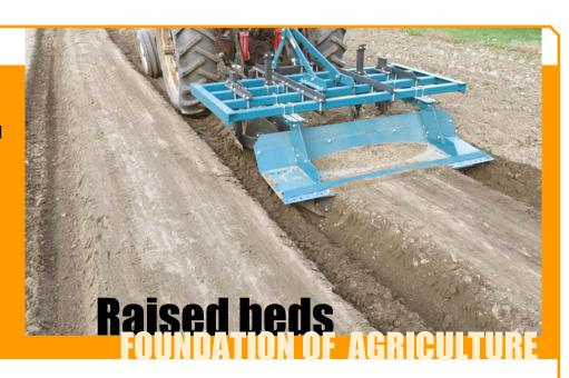
Bed Shapers work in loose prepared soil to form beds from scratch. The shaper pan fills and firms beds behind bed-filling attachments. Bed top width is exact with formed bed sides. Bed height is exact for consistent working depth with plastic mulch layers, planters, drip tape applicators and cultivators.
