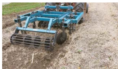
Bed reconditioner working-in cover crops
