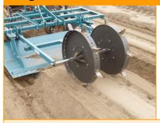
Puncher wheels trailing a Bed Shaper are very practical to get ready to plant. Rows are perfectly aligned for precision cultivation.
