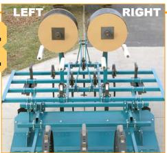
Use (1) 2125-TB and (1) 2125-TBL or (1) 4125-TB and (1) 4125-TBL to install two tape lines for two, three or four row crops. These also feature spool shafts and spool nuts with left-hand thread. Spool shafts point to the rear to set tape rolls close together.
