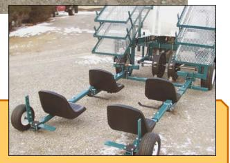
Add 3rd or 4th seat to plant 3 or 4 rows. Also speed-plant 2 rows. Rear gauge wheels provide better support and a better ride. Stacking racks also shown
