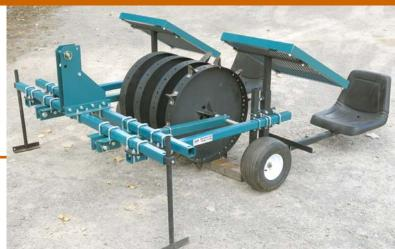
Equip with the number of puncher wheels needed to match your row system. Utilize compact tractors - or larger.
