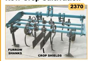
S-tines are effective for mid-to-late cultivation and durable in rocks. Add row crop shields or utilize Beet Knives or Tender Hoes to cultivate up close to the row. Upgrade to heavier Furrow Shanks to loosen compacted wheel tracks.
