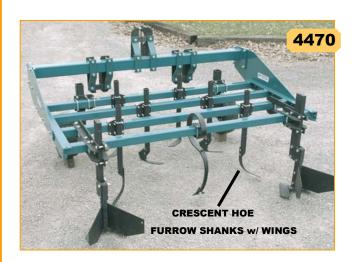
4-bar toolbar frames provide more toolbar space for offset Knives and Sweeps to pass more residue or allow higher ground speeds.
