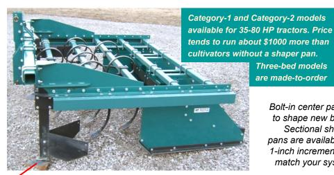
Loosen compaction in furrows. Shanks have shear-bolt safety feature
