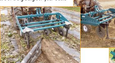
Split mulch down the middle to pull each half away from the row, which is fundamental to roll off soil and debris. The loose plastic on top of the ground can be gathered by hand or rolled up by machine.
