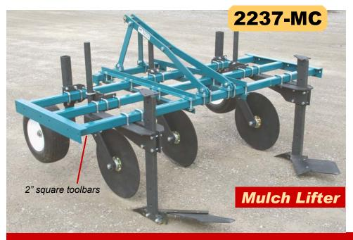
Model 2237-MC is rated similar to the 3117-M but built on a cultivator toolbar. Put the versatile 3-bar frame to work loosening plastic mulch after harvest then again next spring uprooting weeds between mulch rows.
