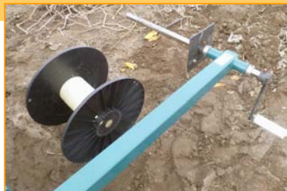
Easy-on, easy-off spool drivers positively engage spool to shaft
