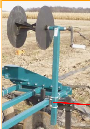
Remove half spool and pull off material bundle
