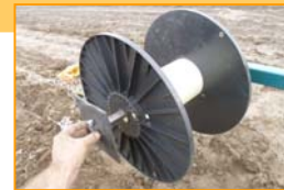
Easy-on, easy-off spool drivers positively engage spool to shaft
