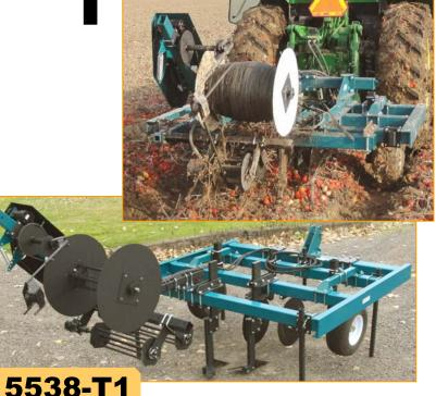
AutoWinder<sup>™</sup> is designed to travel down the row and pull loosened plastic mulch or drip tape from soil and residue. AutoWinder<sup>™</sup> includes state-of-the-art pulling and winding features for fast and efficient operation.
