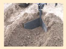
Furrowers can be used as a simple planting tool or to ditch furrows for water drainage at the head of the field
